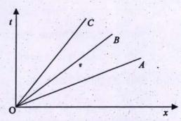
The figure shown above gives the time (t) versus position (x) graphs of three objects A, B and C. Which one of the following is the correct relation between their speeds  $V_A$ ,  $V_B$  and  $V_C$ , respectively at any instant (t > 0)?
