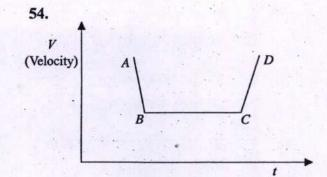
In the given velocity (V) versus time (t) graph, accelerated and decelerated motions are respectively represented by line segments
