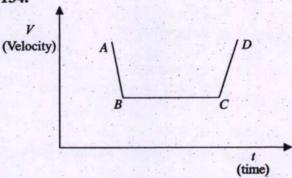
In the given velocity (V) versus time (t) graph, accelerated and decelerated motions are respectively represented by line segments
